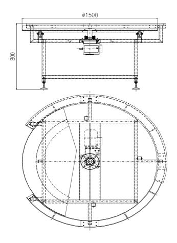
The circular storage table is placed at the end of the conveyer for meat cutting and is used to cut meat sorting. The skeleton is welded from quadratic thin-walled profiles and has adjustable feet. The rotary bowl (Ø 1500 mm) is driven by gear unit and is sandwiched with Orbilan desks.
